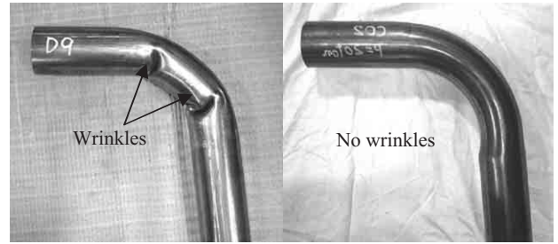
Photo 2 Appearance of bent tube by rotary draw bending and PRB method
